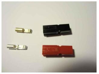
This picture demonstrates the proper orientation of the contacts to the housings. It also shows the proper shape of the contacts prior to installing in the housing. The mating tip must be parallel and straight with the rest of the contact. If it is bent down or up it will not be easy to assemble and may even be impossible to put together
