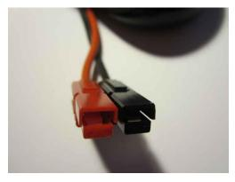
It is wise to assemble the connector housing before inserting the contacts. Do not insert the contacts before crimping or soldering them to the wires. Kind of obvious, but stranger things have happened. The reason for assembling the housings is that particularly with heavier gauge wire, it will be difficult to assemble the housings with the wired contacts already in place. The picture below shows the front end of a properly assembled pair
