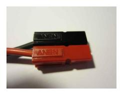
This photo shows the standard layout of a 2-conductor Power Pole Connector. Note that the red or positive connector is always to the right of the black or negative connector with the connectors "top" facing you. The "top" is the wider of the two opposite faces. The "top" is also the only place that Anderson's Logo appears on the housing.
