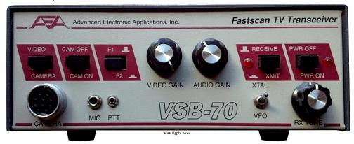
The AEA model VSB-70 is a Fast-Scan Television (FSTV) transceiver that operates on the amateur 420 to 440MHz band. The transmitter features two local oscillator crystal-controlled channels and an output of one watt PEP on sync peaks. Receive operation can transceive or use variable
