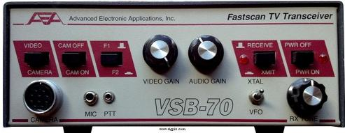
The AEA model VSB-70 is a Fast-Scan Television (FSTV) transceiver that operates on the amateur 420 to 440MHz band. The transmitter features two local oscillator crystal-controlled channels and an output of one watt PEP on sync peaks. Receive operation can transceive or use variable
