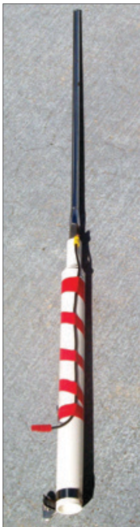
Figure 10 — This "stinger" uses a 10 foot MFJ telescopic whip to extend the mast to 33 feet for use as a vertical antenna. A radial field of many 35 foot radial wires is necessary to make it effective, but the option is there.
