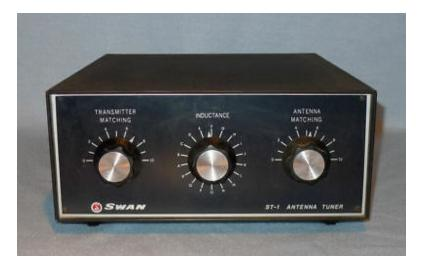
It covers the bands of 160-10 meters, switched inductance T-match type, and is designed as a legal limit (1KW) tuner, built to complement legal-limit amplifiers. Asking price \$100
